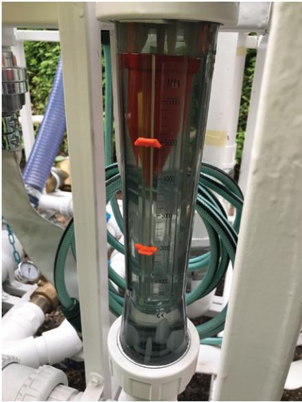
One early morning in May 2019, the A2A and Pipecare teams isolated the first pipe section of a total of three to be treated. Measurements taken by the see-through rotameter were shown to be compatible with the utility's readings of a substantial **8,900 litre/hour** (2.5 litres-per-second ) **aggregate leakage in a 440 meter long section** that was assigned by A2A for treatment.
